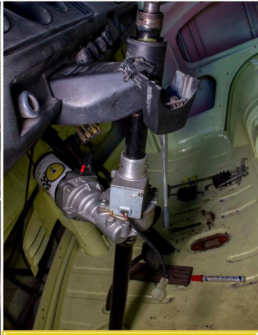
Once the lower portion and EPAS motor are installed, slide the upper column tube into the column bracket and motor housing. Make sure the groove in the upper column is aligned as shown. Once in place, tightened all set screws and re assemble the column mount bracket.
