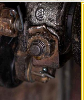
When reconnecting the lower steering shaft to the steering box, be sure to align the groove on the box spline with the bolt hole on the connector.
